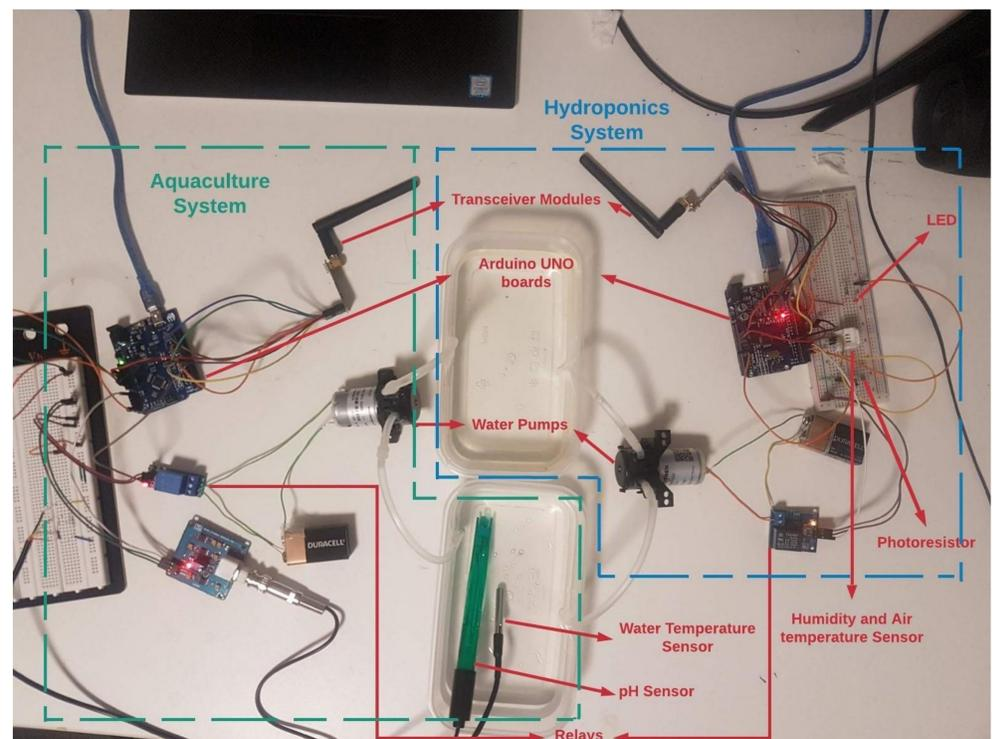
Fig 2 : Assembled System
