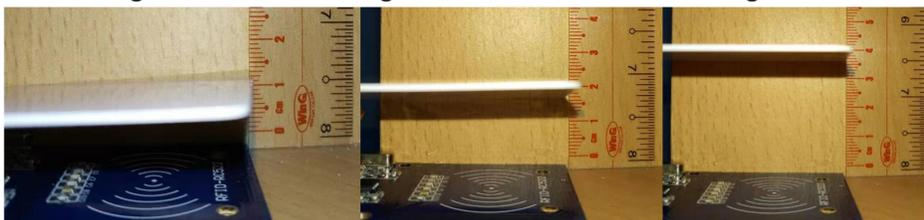
Fig. 3. Read range extended from 1cm to 4cm
