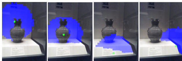
Figure 2. Illustration of the local background sets (blue) for four different candidate regions (green). In this example the neighbourhood radius is r = 200 pixels, and the depth cutoff is t = \sigma/2 . Note that patches lying on salient objects tend to be enclosed by the local background set.
