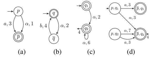
Figure 1: (a)–(b) Weighted automata, representing locally valid plans of components 1 and 2. (c) Projection of (b) on the set of shared actions,  $\{\alpha\}$  (after minimisation). This is message  $M_{2,1}$  (see description of the MPA). (d) Product of (c) and (a), representing the final plan set of component 1. Note the final state cost of 4 in (c)–(d).
