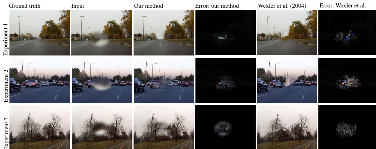
Figure 11. The raindrop removal results using our methods and the method of Wexler et al. [21].
