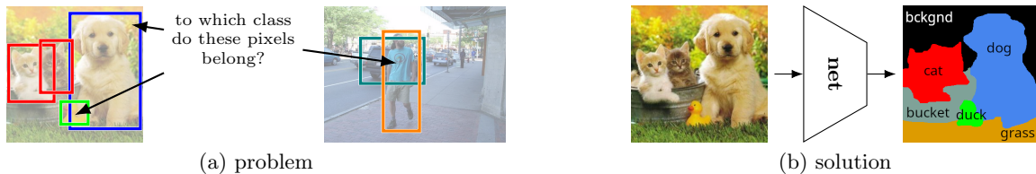
Figure 69: One problem with object detection is that it does not fully specify which pixels belong to each object found in the scene (left). A proposed solution is semantic segmentation—annotate every pixel in the image with a category label (right).
