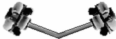
**Figure 2.1.1:** Simple omni-wheeled system with angled universal wheels.
