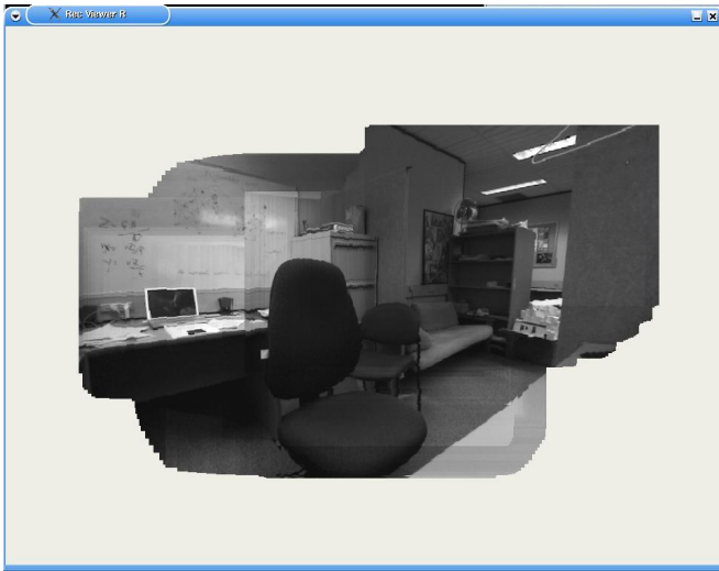
Fig. 3. Snapshot of online output of the active rectification process: mosaic of rectified frames from right CeDAR camera. The full video sequence is also available (Section X).
