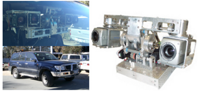
Fig. 2. The research platform. Left: The Smart Car (bottom) and CeDAR mounted behind the windscreen (top); Right: CeDAR .
