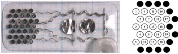
Figure 1: The intraocular electrode array comprises a silicone substrate (19 mm long, 8 mm wide) with 33 platinum stimulating electrodes (30 x 600  $\mu\text{m}$ , 3 x 400  $\mu\text{m}$ ), and 2 large return electrodes (2000  $\mu\text{m}$ ). The outer ring of electrodes (shown in black, right) was connected together to form a “guard ring” return electrode. Stimulating electrodes were arranged in a hexagonal configuration, with uniform distance of 1 mm between neighboring electrode centroids.
