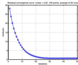
Figure 4. An average convergence curve of the alternation procedure, i.e., residual error v.s. number of iterations. The curve was generated by averaging 50 tests with 0.05 degrees std noise.
