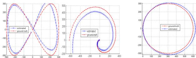
Figure 10. *Measured ground-truth trajectories vs. recovered trajectories. From left to right we test three different type of curves, an  $\infty$ -shaped curve, a spiral and a circle. Each sequence has 101 frames.*
