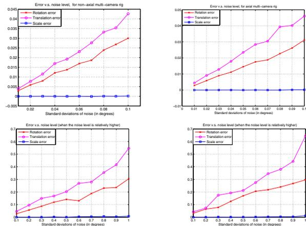
Figure 6. This figure shows estimation accuracy (in rotation, translation, scale) as a function of noise level. The error in scale estimate is defined as  $1 - \frac{\|\hat{t}\|}{\|t\|}$ . Top row left: results for simulated non-axial camera rigs; Top row right: results for simulated axial camera rigs. Bottom row shows the same results as in the top row, but with much higher levels of noise.
