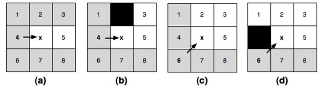
Figure 2: We show several cases where a node  $x$  is reached from its parent  $p(x)$  by either a straight or diagonal move. When  $x$  is expanded we can prune from consideration all nodes marked grey.
