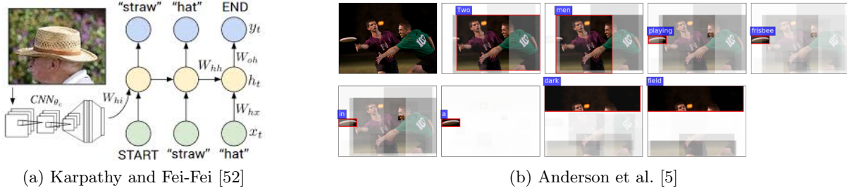
Figure 90: Image captioning models combine a CNN image encoder with an RNN language decoder.
