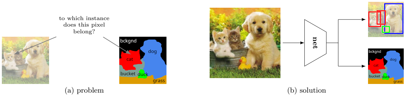
Figure 77: One problem with semantic segmentation is that it does not distinguish between instances of the same class (left). A proposed solution is instance segmentation—perform object detection and semantic segmentation jointly (right).
