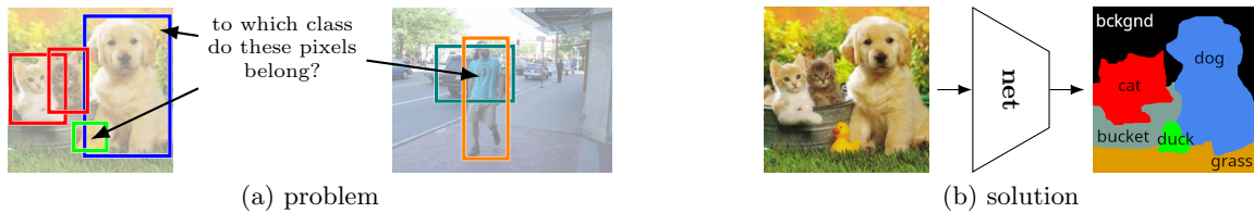
Figure 69: One problem with object detection is that it does not fully specify which pixels belong to each object found in the scene (left). A proposed solution is semantic segmentation—annotate every pixel in the image with a category label (right).
