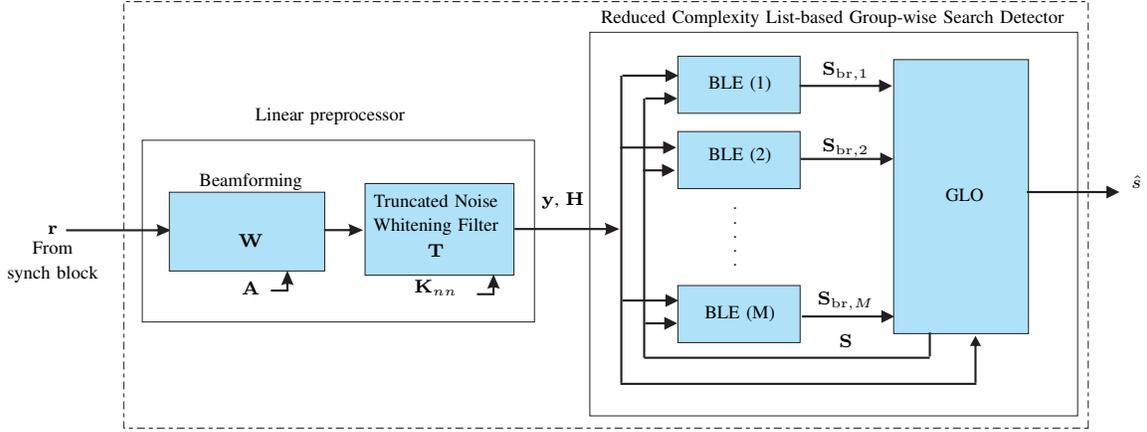
Fig. 3. The block diagram of the proposed receiver. BLE: Branch list estimator. GLO: Global list optimizer.
