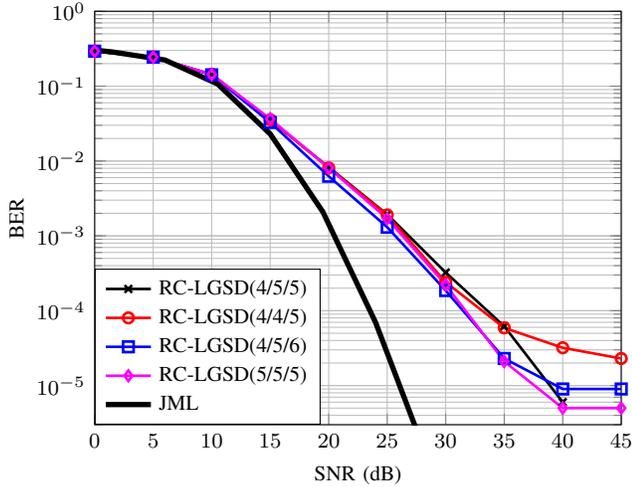
Fig. 5. Performance of 16APSK using different iteration sets.
