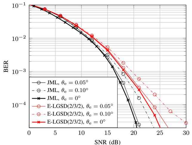
Fig. 8. Pointing error effect on 8PSK BER, for error angle  $0.05^\circ$  and  $0.1^\circ$ .
