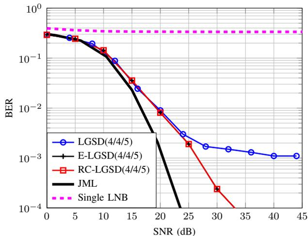
Fig. 7. Performance of 16APSK using different detectors.
