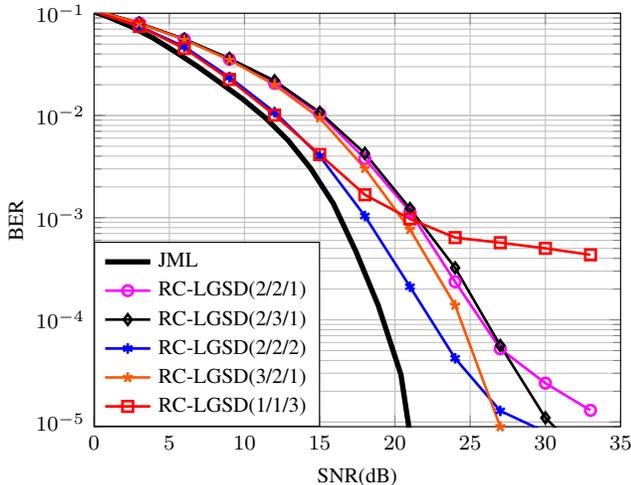
Fig. 4. Performance of 8PSK using different iteration sets.
