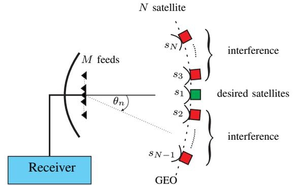
Fig. 1. The system setup for  $N$  satellites in the geostationary orbit, and  $M < N$  LNBS. The dish is directed to the desired satellite,  $s_1$ .
