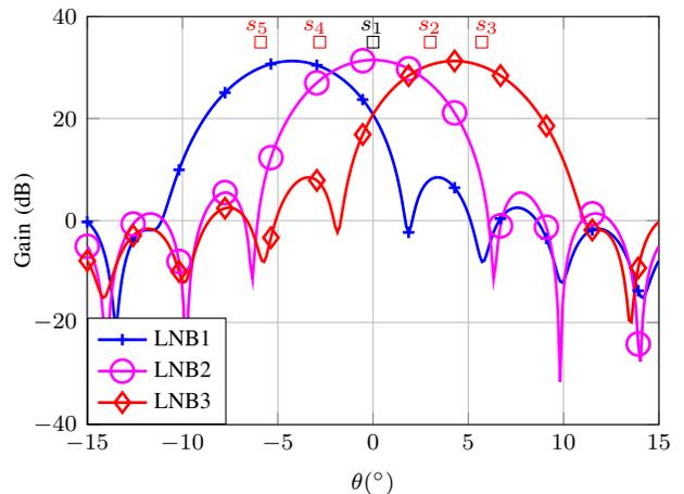
Fig. 2. Radiation patterns of three LNBs mounted on a 35-cm dish.
