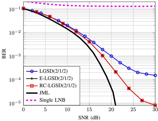
Fig. 6. Performance of 8PSK using different detectors.
