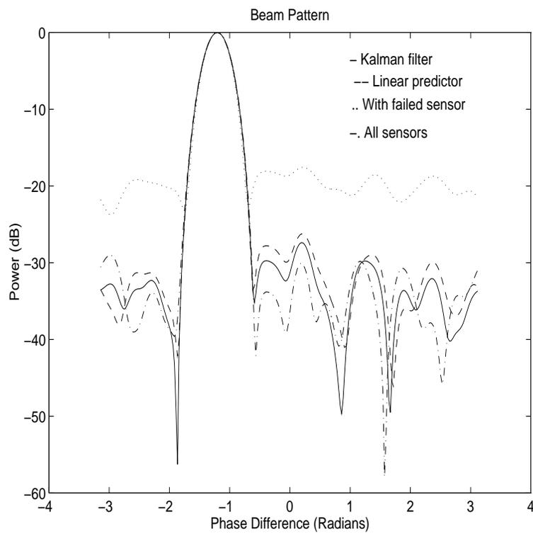
Fig. 3. Normalized Beam Power versus Phase Difference for SNR 10dB
