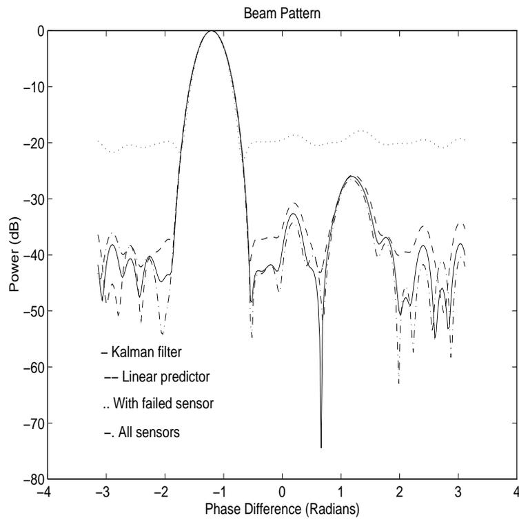
Fig. 2. Normalized Beam Power versus Phase Difference for SNR 20dB
