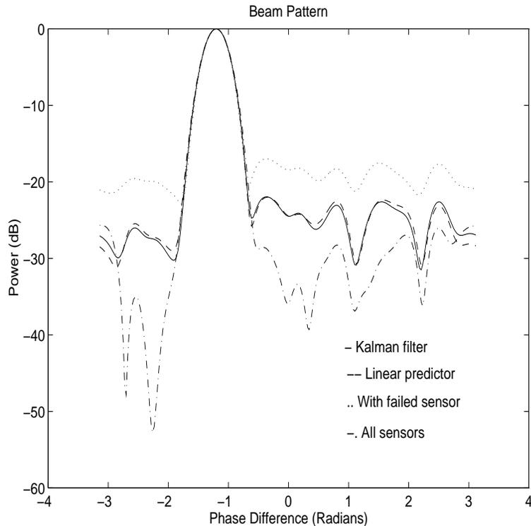
Fig. 4. Normalized Beam Power versus Phase Difference for SNR 3dB
