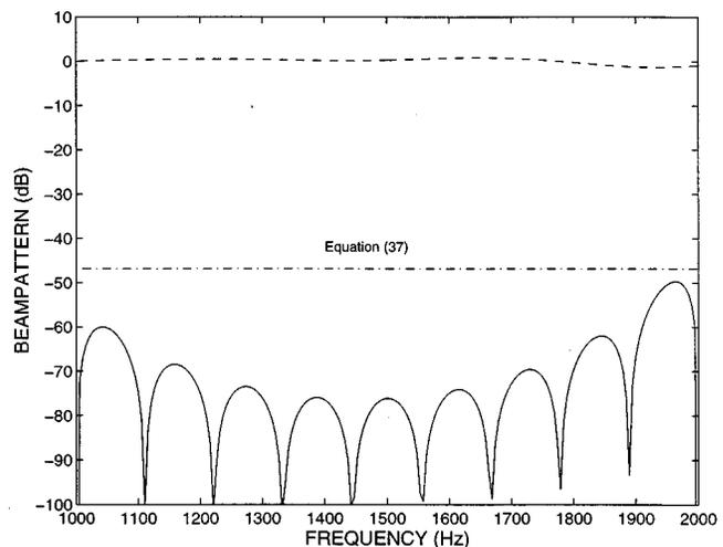
FIG. 8. Array responses of quiescent design (--) and multiple frequency null design (—) at the null direction ( $\theta=30^\circ$ ) over the array design frequency band. The predicted null depth from Eq. (37) for the multiple frequency nulling approach with  $M=10$  is also shown (-.-).
