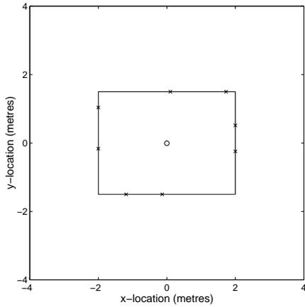
Figure 1: Location of sensors ( $\times$ ) and source ( $\circ$ ) within a  $3 \text{ m} \times 4 \text{ m}$  room.
