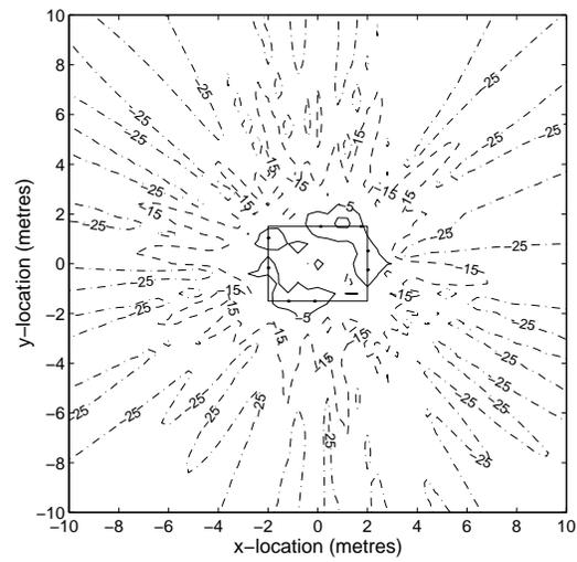
Figure 2: Response of the designed beamformer. The source is located at  $\mathbf{s} = [0, 0, 0]^T$ , and the sensors are located at the positions denoted by the small dots. The gain at  $\mathbf{s}$  is 0 dB.
