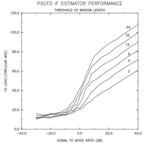
Figure 3: Dispersion of the PSCFD estimator against signal-to-noise ratio for various window lengths.
