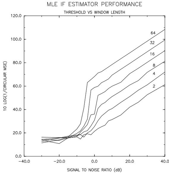
Figure 2: Dispersion of the ML estimator against signal-to-noise ratio for various window lengths.
