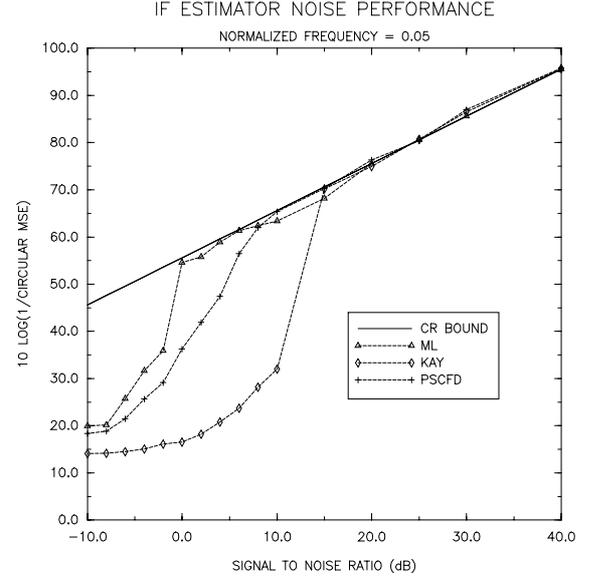
Figure 1: Comparison of the dispersion of the ML, PSCFD and Kay estimators against signal-to-noise ratio for a normalized frequency of 0.05. The window length  $M = 47$  for the ML estimator and the smoothing window length  $P = 45$  for the PSCFD and Kay estimators.
