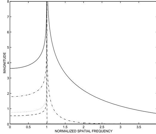
Figure 1: Magnitude of the Fourier transform  $S_{r,\theta}(\xi)$  of the signal  $s_{r,\theta}(x)$  for  $r = 3.5\lambda$ ,  $\theta = 1$  degrees (solid line);  $r = 3.5\lambda$ ,  $\theta = 5$  degrees (dashed dot line);  $r = 3.5\lambda$ ,  $\theta = 90$  degrees (dashed line) and  $r = 100\lambda$ ,  $\theta = 1$  degrees (dotted line) plotted against the normalized spatial frequency  $\xi/k$ .
