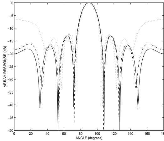
Figure 2: Magnitude of the array response of a  $\lambda/2$  spaced 7 sensor array (dotted line),  $\lambda/4$  spaced 13 sensor array (dashed line) and  $\lambda/6$  spaced 37 sensor array (solid line) to a nearfield source at  $3.5\lambda$  from the array origin. Aperture length of each of three arrays are equal to  $3\lambda$ .
