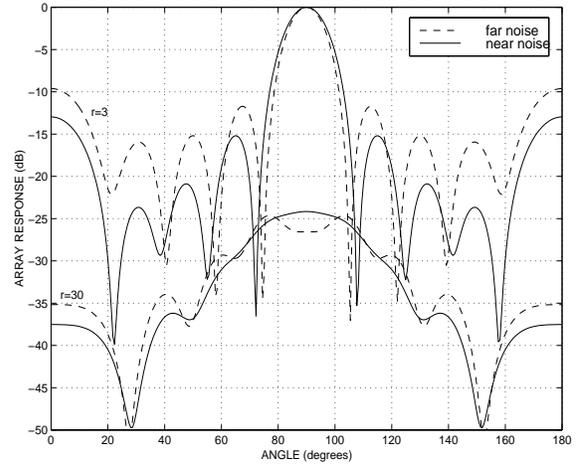
Figure 1: Response of the optimum array based on nearfield noise model (solid line) to sources at 3 and 30 wavelengths from the array origin. Also shown is the response of the farfield noise model based array response (dashed line).
