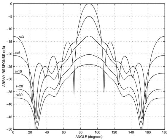
Figure 2: Response of the optimum array (nearfield noise model) at 3, 5, 10, 20 and 30 wavelengths from the array origin
