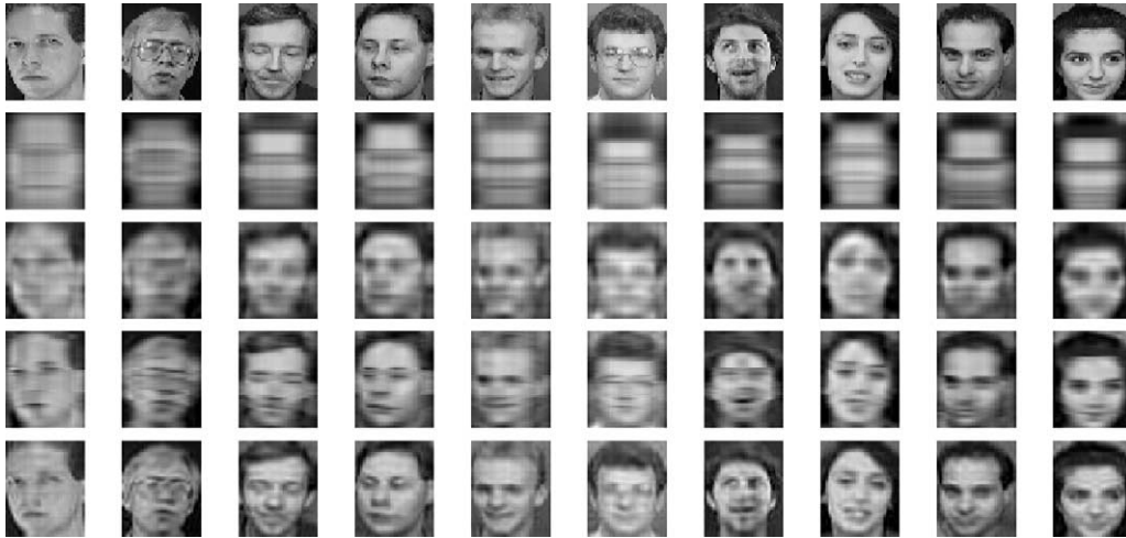
Fig. 7. First row: raw images. Second row and fourth row: image reconstructed and compressed by 2DPCA using 2 and 8 principal component (vectors), respectively. Third row and fifth row: image reconstructed and compressed by B2DPCA with d=10 and d=20 , respectively.
