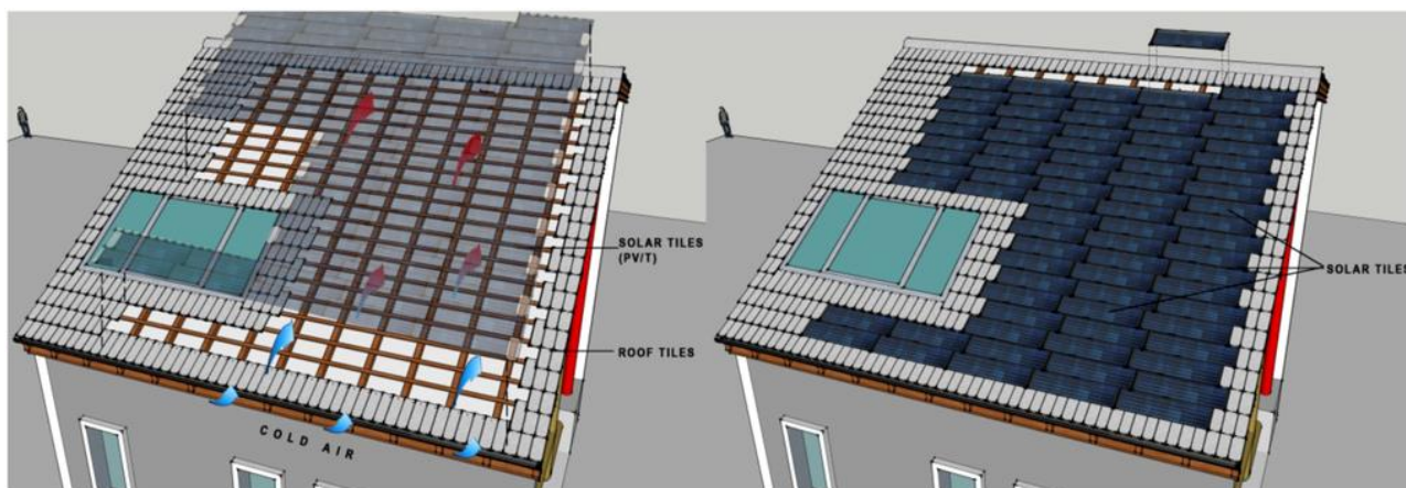
Figure 5: Example mounting for a Hybrid PVT system. Source: Noguchi, 2013.
