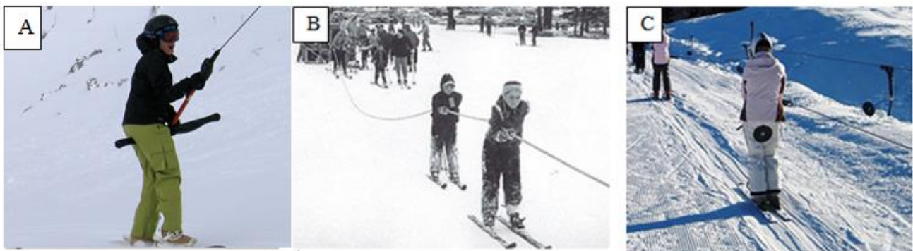
Figure 1: Typical Australia ski resort surface lift types [A] A T-bar (Tan, 2012) [B] A rope tow (Anon., 2012) [C] a J-bar lift (Frank, 2013)
