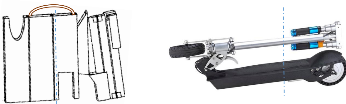
Figure 5 - Comparison of balance points of the new (left) and old (right) scooter designs when folded
