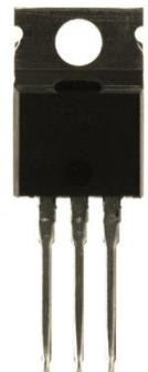
Figure 10 - IRFB4115 TO-220 MOSFET as used in the scooter
