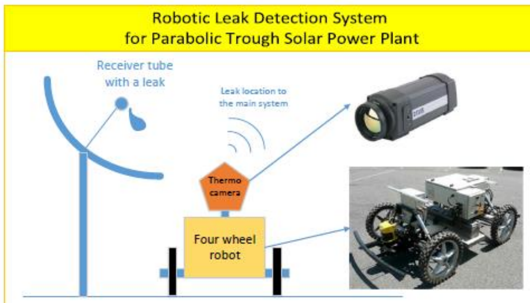
Figure 1. Recommended leak detection system from ENGN2225.
