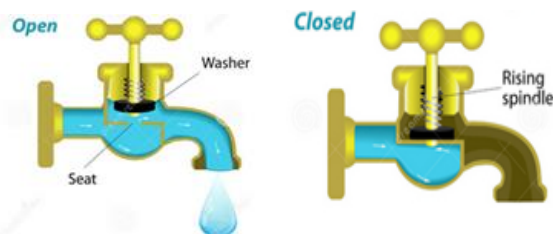
Figure 2: Mechanism Diagram of Water Tap (Anderson, 2008).
