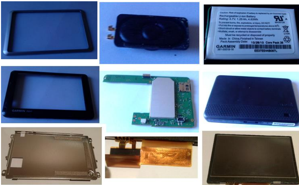
Figure B.2: The components of the Garmin Nuvi 1350 (2009).
