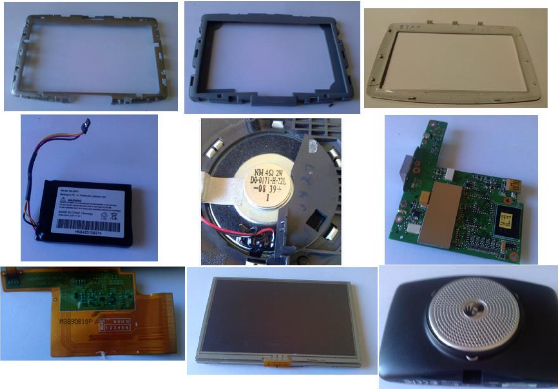
Figure B.1: The components of the TomTom XL 310 (2007).
