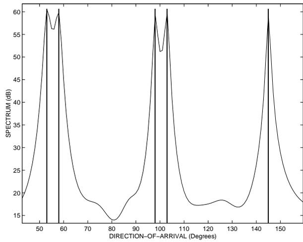
**Figure 1.5:** The estimated spatial spectrum of the Multigroup sources using algorithm of [4]
