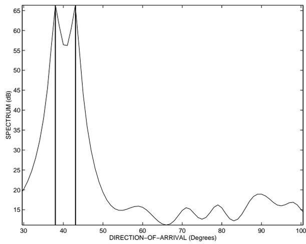
**Figure 1.2:** The estimated spatial spectrum of the correlated sources using the algorithm of [2].
