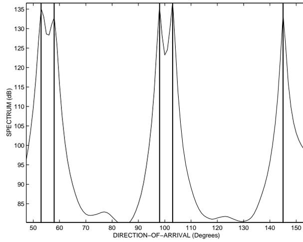
**Figure 1.7:** The estimated spatial spectrum of the Multigroup sources using Modal Space Processing for a wider frequency band [300 : 3000]Hz. )
