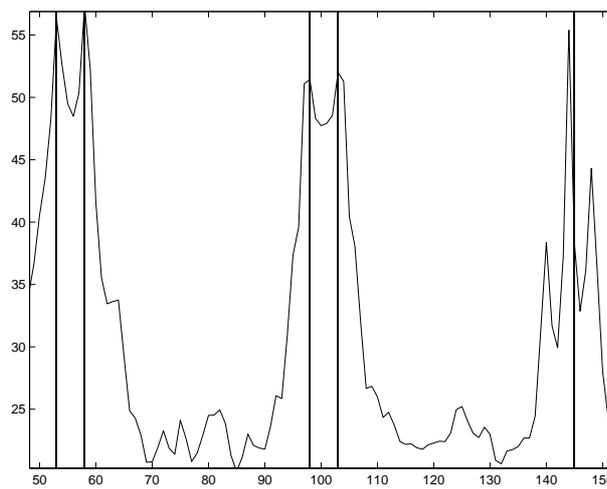
**Figure 1.8:** The estimated spatial spectrum of the Multigroup sources using algorithm of [4] for a wider frequency band [300 : 3000]Hz.
