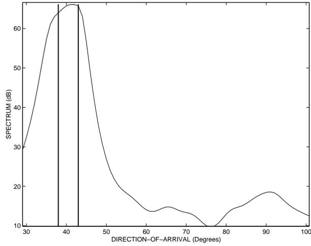
**Figure 1.4:** The estimated spatial spectrum of the correlated sources using prior angle estimation of  $53^\circ$ .
