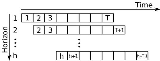
Figure 1: A receding horizon market considers the exchange of power over a forward horizon of  $T$  time steps, which recedes as the first time step is reached in real-time. The market clears each horizon, but agents only need to commit to the outcome of the first time step in each horizon.
