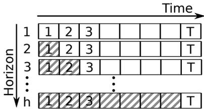
Figure 2: Representation of the TRH horizons. Shaded areas represent the time steps in which variables are constrained to take on values from the previous horizon (according to equation (4)).
