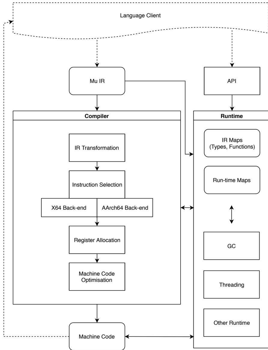
**Figure 2.2:** An overview of Zebu VM, illustrating important components and interaction between them. Dotted lines illustrate how Zebu fits in a language implementation.
