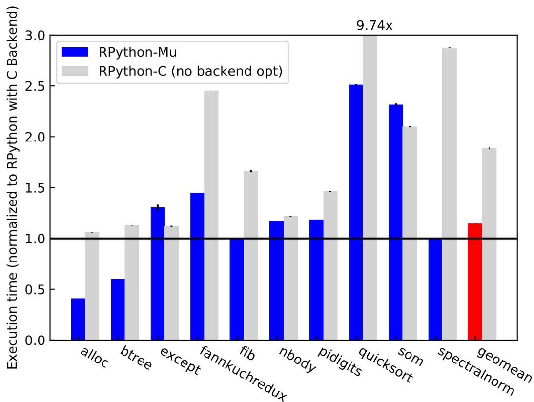
**Figure 5.3:** Performance of RPython-Mu (lower is better). The baseline and the RPython-C (no back-end opt) results illustrate a range of how back-end optimizations affect the overall performance for the C back-end. RPython-Mu results show our compiler performance.
