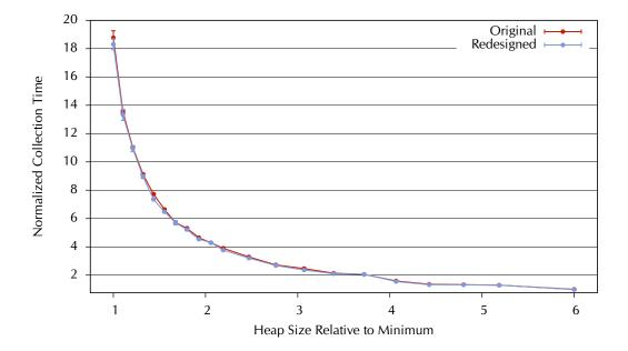
**Figure 8.2:** Garbage collection performance for the *full-heap mark-sweep* configuration before and after the redesign.
