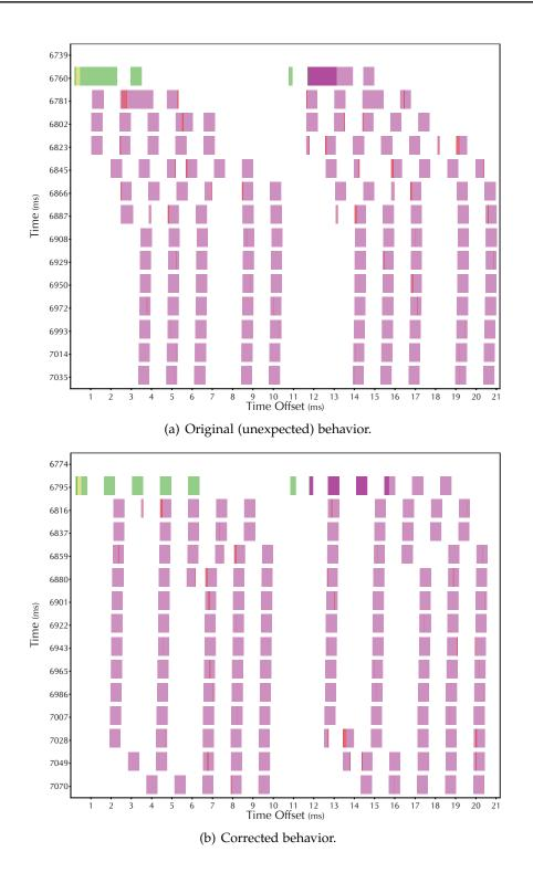
**Figure 9.3:** Oscilloscope view of unexpected and expected scheduling of collector quanta (colors indicate the type of collection activity occurring, which is not relevant to this discussion).
