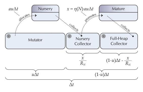
**Figure 5.7:** Time dilation due to generational collection causes additional allocation during a major heap collection, but attenuates all allocation by the survival rate  $\eta(N)$ .
