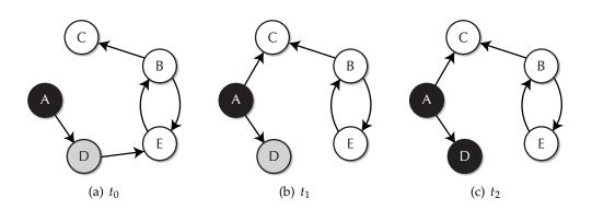
Figure 4.2: Adding a cycle to the mutator–collector race.
