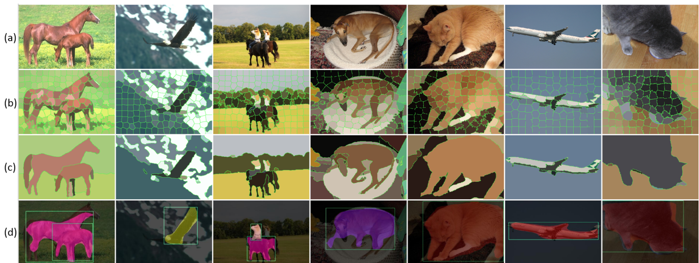
Fig. 4. (a) images, (b) and (c) superpixel regions and edge regions. Pixels in each region are replaced with their mean color, (d) masks generated by MNC [40]. (i) We can see that edges divide images into fewer regions than superpixels and thus preserving more compactness of objects, which is helpful for saliency prediction. (ii) The superpixels and edges regions achieve higher boundary accuracy than masks generated by MNC [40]. Best viewed in color.
