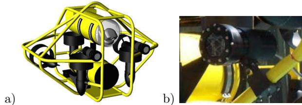
Figure 1: a) *Kambara*, the autonomous underwater vehicle at the Robotic Systems Lab, ANU. b) Camera mounted in a water-tight enclosure.
