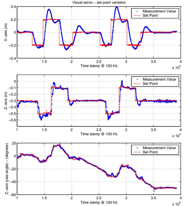
Figure 3: Experimental result in visual servo on a fixed target. This figure shows result of movements in square on  $x-z$  plane as illustrated in Figure 4.
