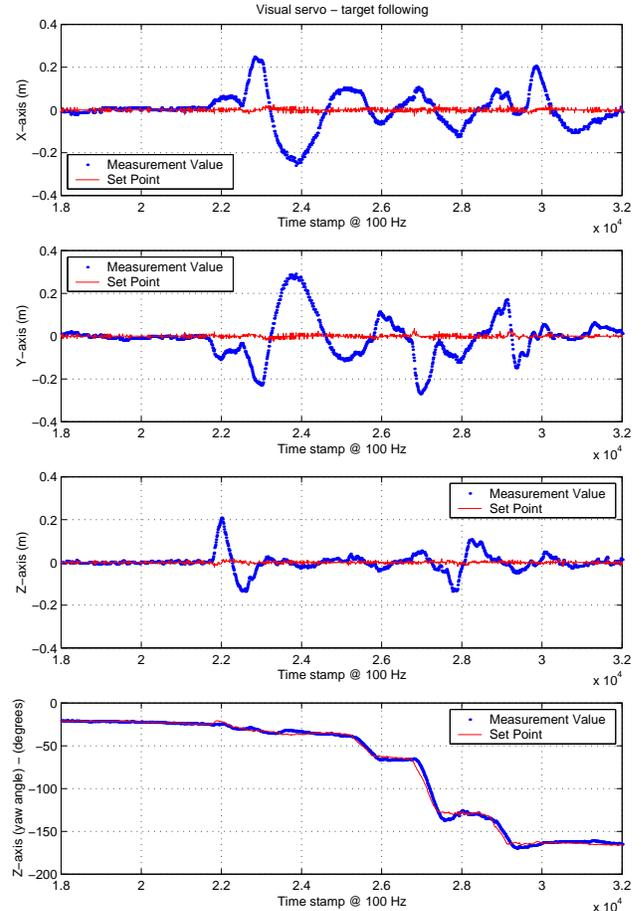
Figure 5: Experimental result in visual servo on a moving target. This figure shows the result of following a target that moves in a circular pool. The diagram of the target movements is illustrated in Figure 6.
