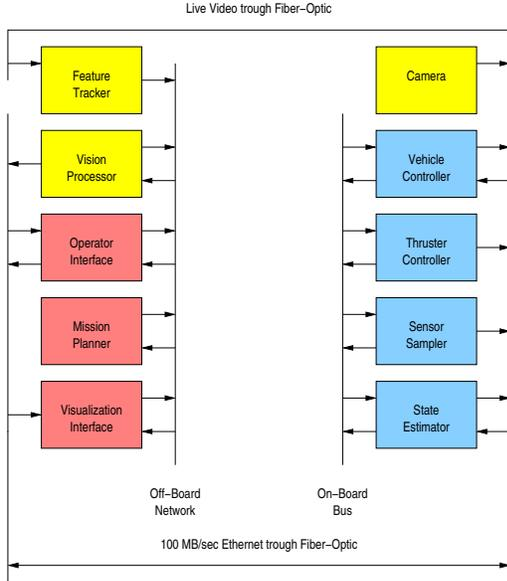
Figure 2: Software architecture of on-board and off-board modules.
