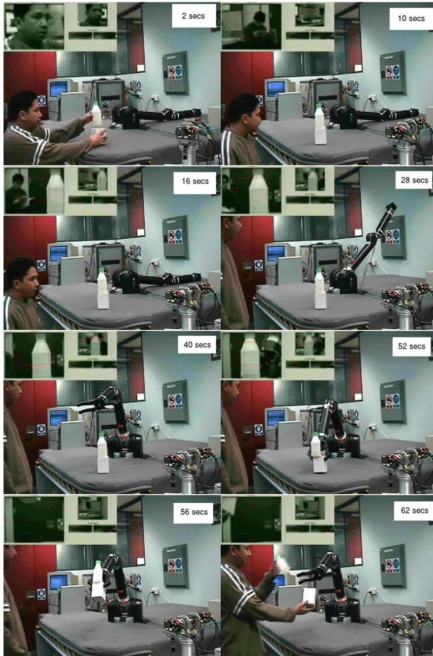
**Fig. 8.** Human-robot interaction experiment: A user instructs the WAM to pick up and hand over the object he is looking at. The object of arbitrary size, shape and color is placed on an unknown position in robot workplace. Upper left inset shows images from the cameras.
