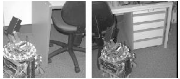
Figure 23. Some environment features that are hard for a sonar ring to detect.
