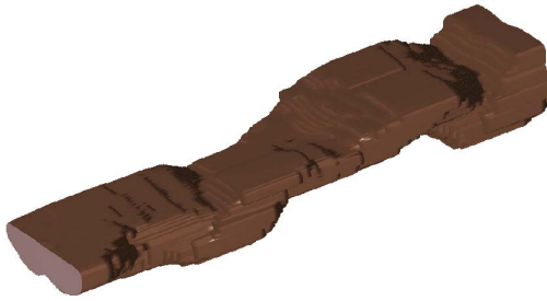
Figure 14: Part of a segmented fiber ( 200 \mu\text{m} length), which was identified by MSER tracking.
