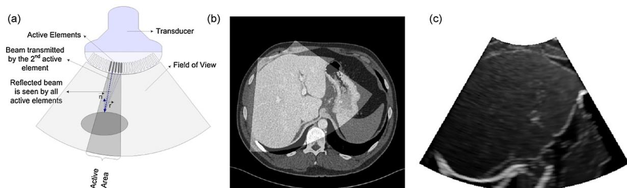
**Fig. 1 – (a) Schematic of a convex array transducer with a multi-element active aperture; (b) ultrasound field of view superimposed on the liver of a human subject; (c) our simulated ultrasound (combined reflection and scattering images), for the region of interest shown in (b). Also notice shadowing on the right-hand side due to an air–tissue interface and in the middle–bottom of the image due to a bone–tissue interface.**
