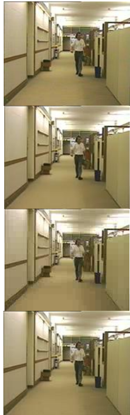
Fig. 9. "Hall Monitor" frame #264 (a) original; (b), (c) and (d) reconstructed after being encoded respectively by H.264 (0.12 bit/pixel), FHVC (0.12 bit/pixel), and FHVC (0.3 bit/pixel).
