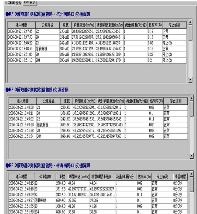
Fig. 11 The measured speed of urban-bus for its historical event evaluates the result for every 5 minutes.
