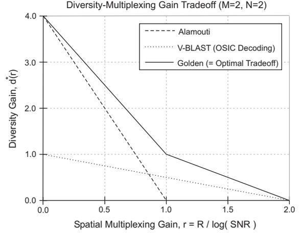
Fig. 2. Diversity-Multiplexing Gain Tradeoff (M=2, N=2) [10][11]
