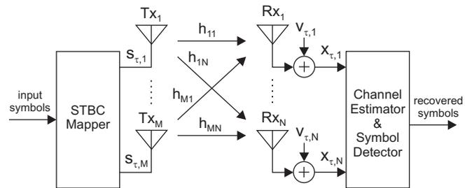
Fig. 1. MIMO communications system model
