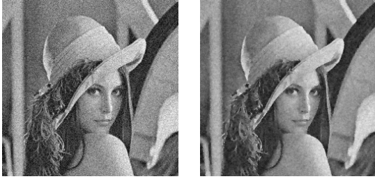
Figure 7. The corrupted input image was created by adding Gaussian noise ( \sigma = 4 labels) to a 256 \times 256 image quantized to 64 labels/grey levels. A truncated convex function was used for both the data and smoothness terms. The enhancement of LazyElimination is shown on the right. All algorithms were run for three iterations, and each produced a similar solution.
