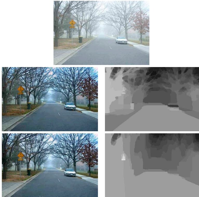
Fig. 7. The foggy input image (top) is enhanced using the contrast data measure. The estimated depth of the parked car is wrong (since the appearance of the car is too similar to that of the fog to provide reliable information). The monotonic preference (bottom row) improves the enhancement.
