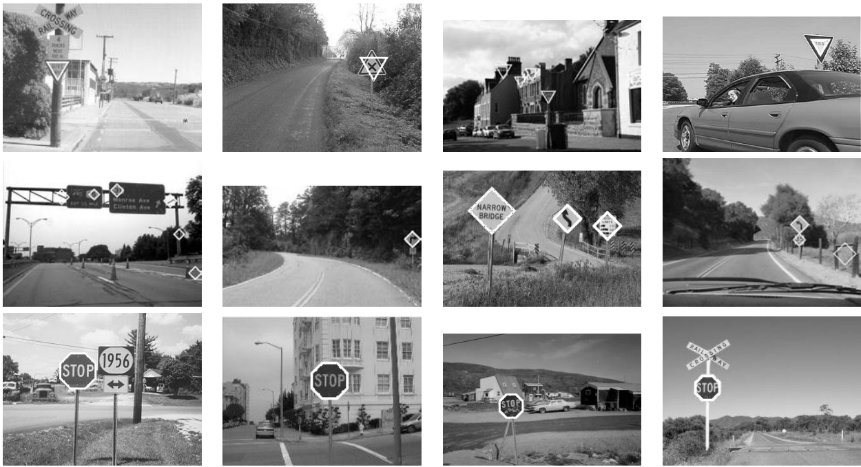
Fig. 8. Results for searching for triangles (top row) with r \in \{8, 10, \dots, 18\} , and squares (middle row) and octagons (bottom row) with r \in \{10, 12, 14, 17, 20, 25\} . All targeted signs are correctly detected.
