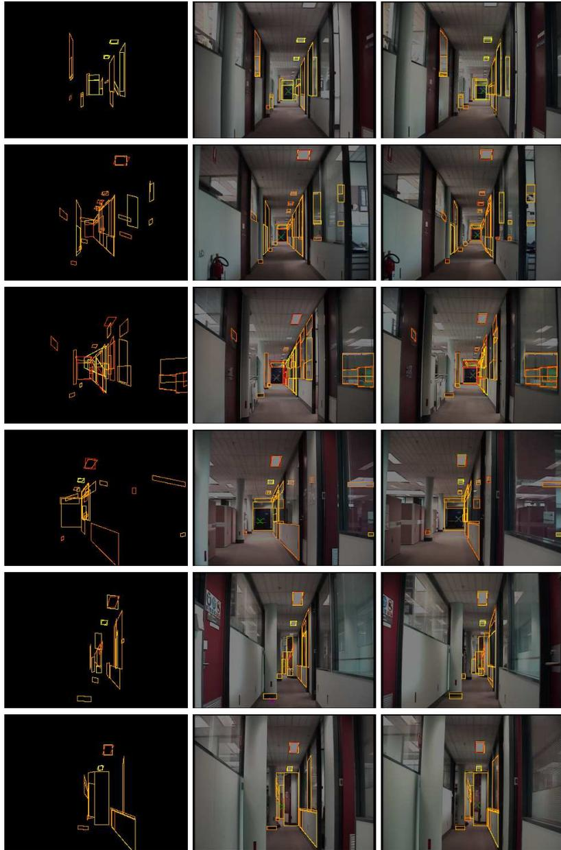
**Fig. 4.** Matching perspective rectangle features in a corridor sequence, samples taken from the 1000 frames in the video sequence. Centre and right pictures show matched features in the image. Left pictures show 3D rectangle features viewed from a ‘virtual camera’
