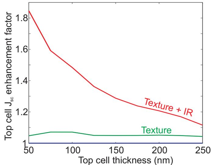
Fig. 3.  $J_{sc}$  enhancement factor for each cell structure vs. top cell thickness. This factor is the ratio of the top cell  $J_{sc}$  of a given structure to the  $J_{sc}$  of the planar cell at equal top cell thickness
