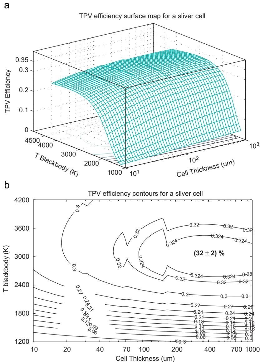
**Fig. 7.** (a) Sliver cell efficiency surface and (b) sliver cell efficiency contour map. A broad efficiency maximum for *large* cell thickness is observed. The small discontinuities are an artifact resulting from progressively changing the material resistivity to ensure high IQE.
