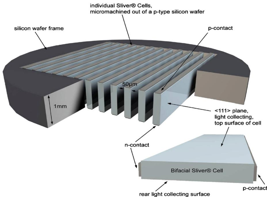
Fig. 2. Diagram of sliver cell fabrication [7].
