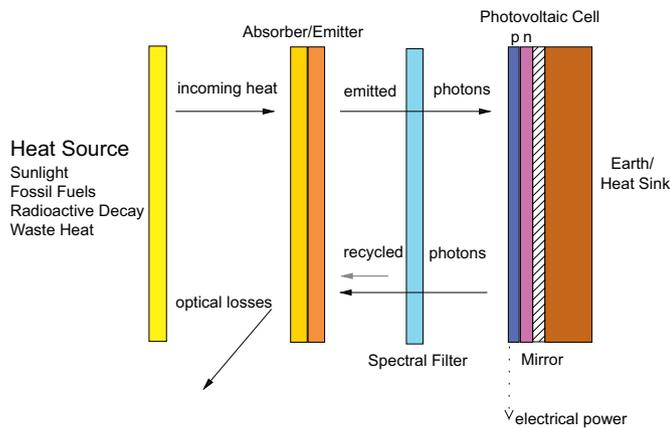
Fig. 1. Schematic diagram of a thermophotovoltaic system.
