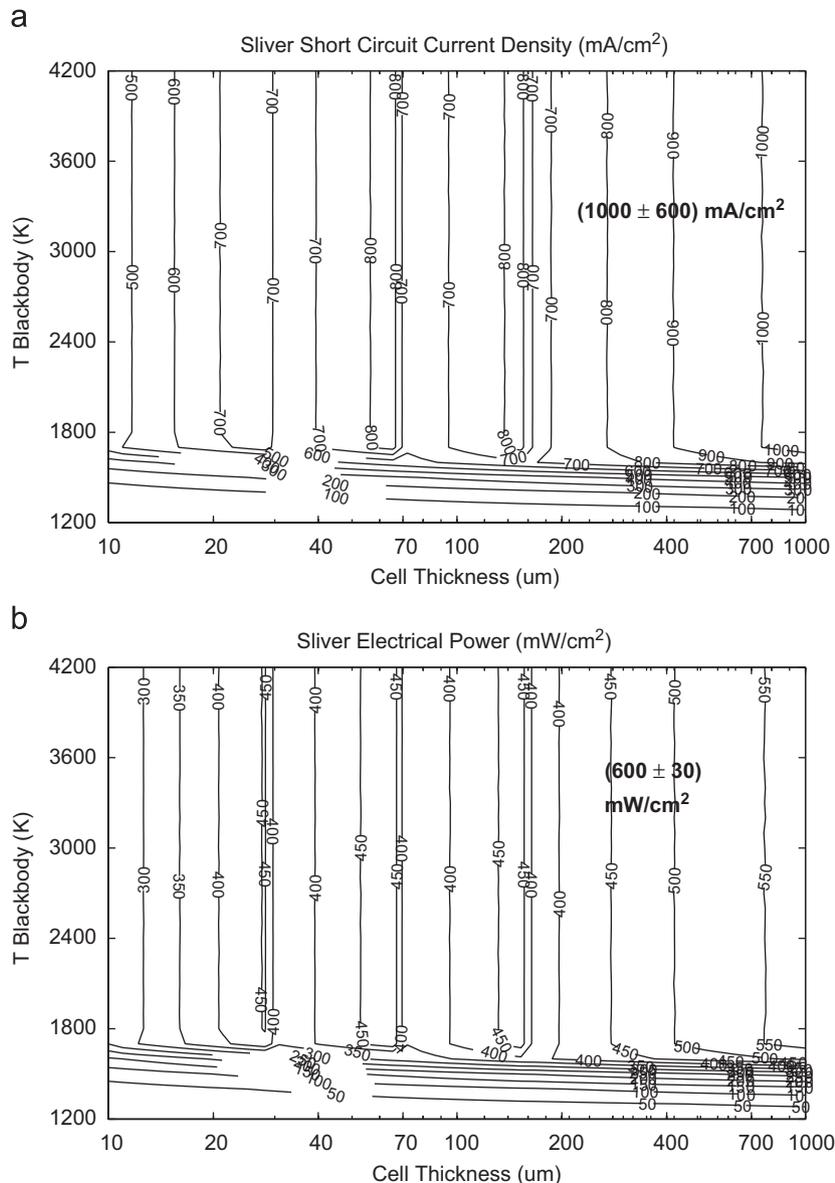
**Fig. 8.** (a) Sliver cell TPV short-circuit current density and (b) electrical power output density. The relatively broad maximum is due to sliver cell performance being limited by cell width, which were held constant at  $300 \mu\text{m}$  for all cell thicknesses. The maximum for *large* cell thicknesses is due to resistive losses being inversely proportional to cell thickness.
