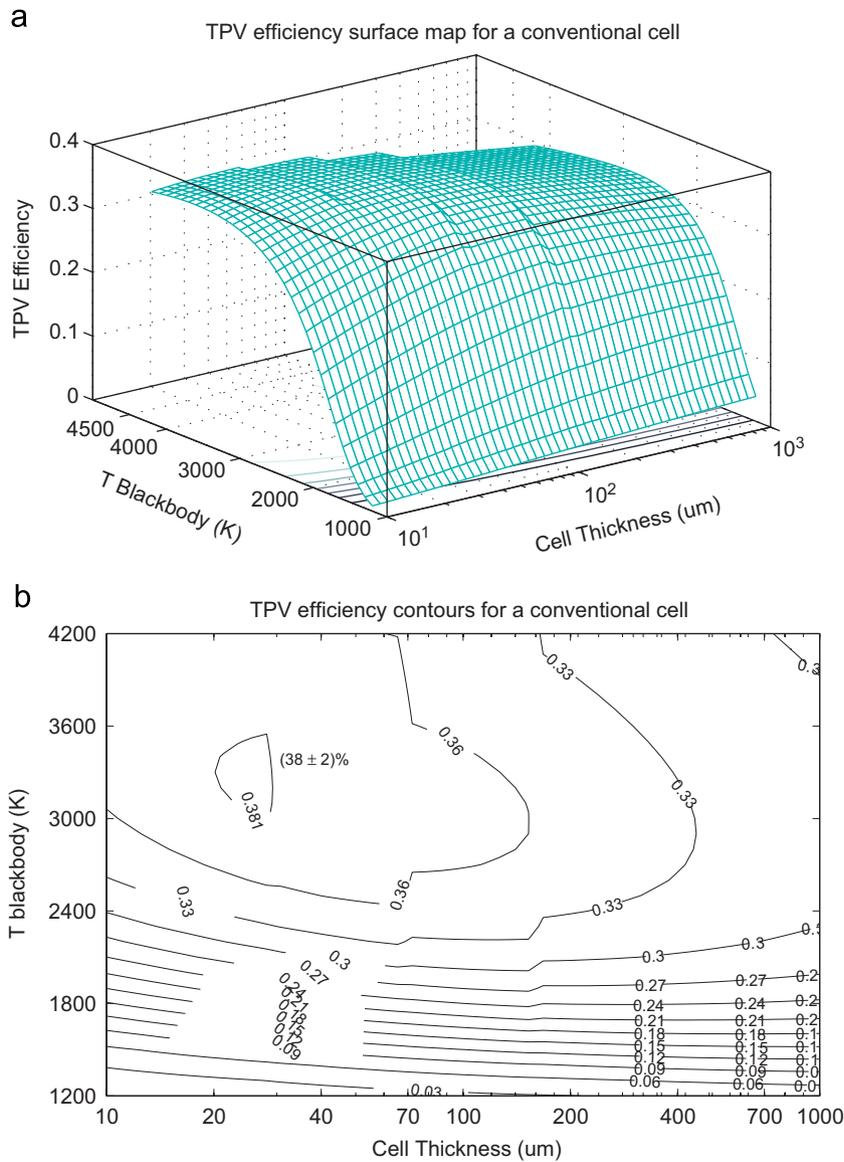
**Fig. 5.** (a) Conventional cell TPV efficiency surface. (b) Conventional cell TPV efficiency contour map. A broad maximum for low cell thicknesses and relatively high blackbody temperatures is observed. The small discontinuities are an artifact resulting from progressively changing the material resistivity to ensure high IQE.
