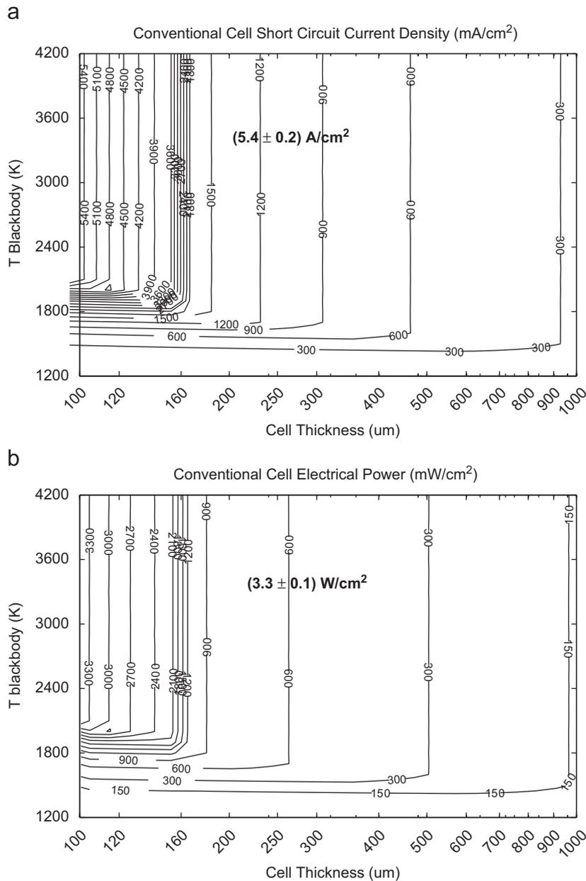
**Fig. 6.** (a) Short-circuit current density and (b) electrical power output densities for a conventional cell in a TPV system. High output power densities are observed for thin cells.
