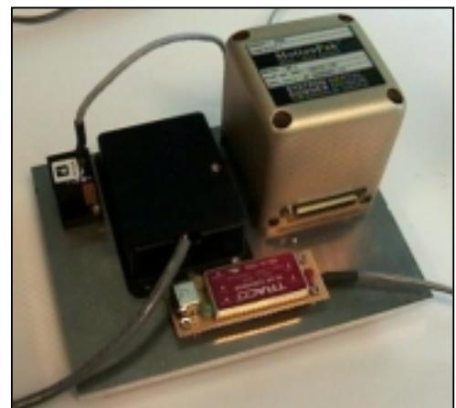
Figure 3.5: Sensors and DC-DC converter mounted fixed onto mounting plate.
