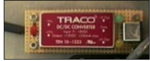
Figure 3.7: DC-DC converter for MotionPak sensor.
