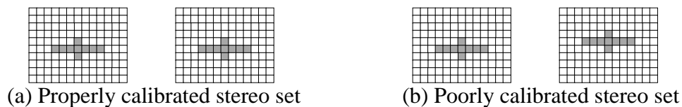
Figure 25 - Calibration of stereo cameras
