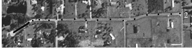
Fig. 12. Handling of road junctions. Black dots are the detected road axis points. Junction 1 was jumped over, while the tracking stopped at junction 2.
