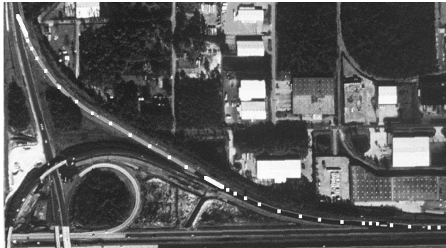
Fig. 7. Road tracking from upper left to lower right. White dots are the detected road axis points, white line segment shows the location of human input.
