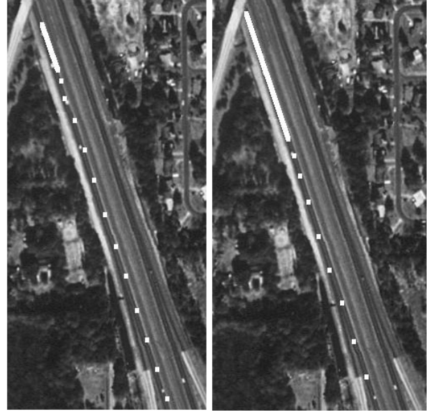
Fig. 11. Example of accurate and inaccurate tracking on the same road. White line segments are the inputs from two users and white dots are the detected road axis points. In the left image, the input is not at the center of the road. It generates a biased road profile predictor, which in turn makes inaccurate road tracking that is deviated from the true road centerline. The right image shows an accurate road tracking initialized by an accurate human input.
