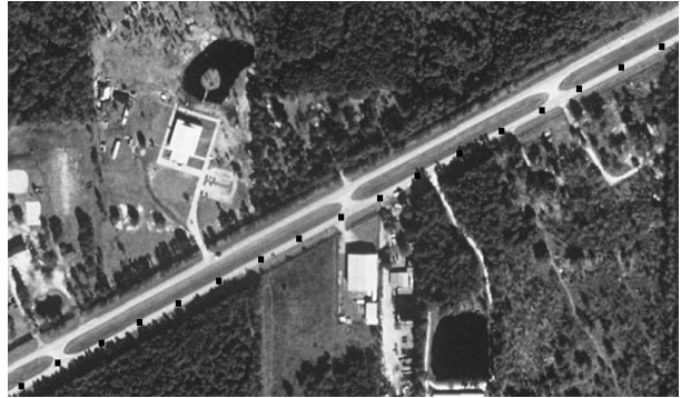
Fig. 8. Example of road tracking. Road tracking proceeds from the upper right to the lower left corner of the image. Black dots are automatically detected road axis points. The tracking is robust when facing occlusions on the road.
