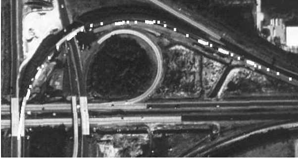
Fig. 12. Example of low efficient road tracking caused by complex road condition. The road tracking starts from the lower left corner of the image. White line segments are the human input and white dots are the tracking result. Due to the complexity of the road, intensive human input is required.
