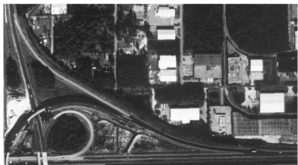
Fig. 1. An image sample of size 663 by 423 pixels extracted from an orthorectified aerial photo. Notice that the occlusions, crossings, and the change in road surface materials lead to abrupt changes in road appearance.
