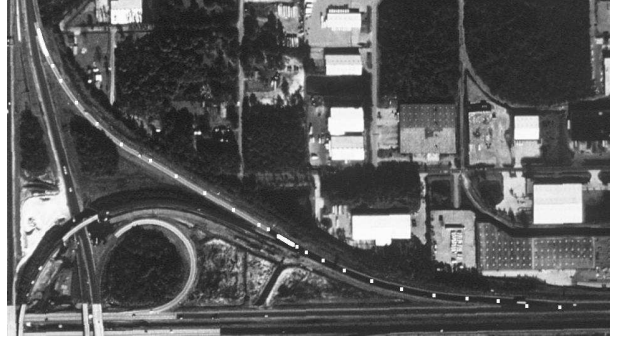
Fig. 7. Example of road tracking. Road tracking starts from the upper left area of the image. White line segments show the locations of human inputs; white dots are the detected road axis points. When the road changes from light to dark, a human input is required to guide the tracking because the dark road has not been experienced by the road tracker.
