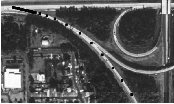
Fig. 9. Example of handling a junction. Road tracking starts from the upper left corner of the image. The black line segment is a human input and black dots are the tracking result.
