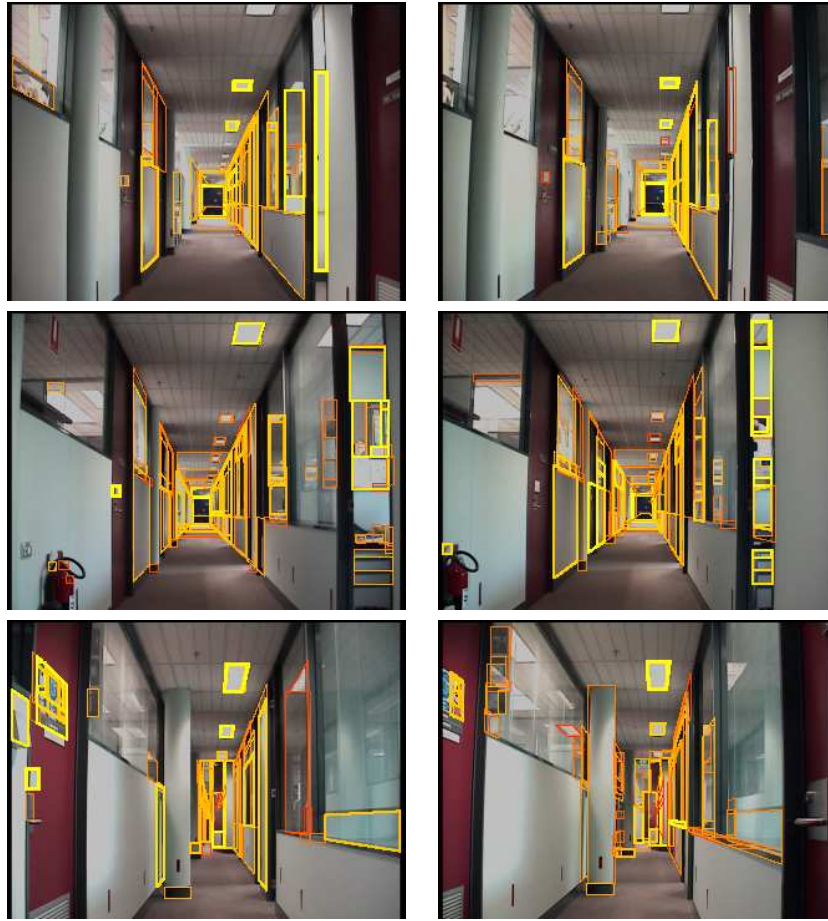
Figure 6: Perspective rectangle features in a corridor sequences.
