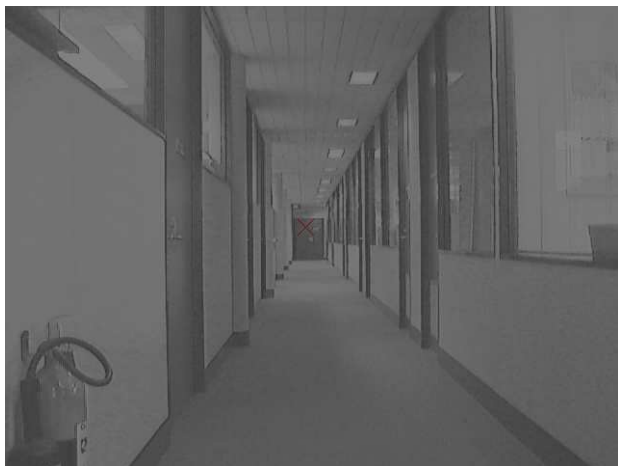
Figure 5: Vanishing point detector. 'X' marks the detected vanishing point
